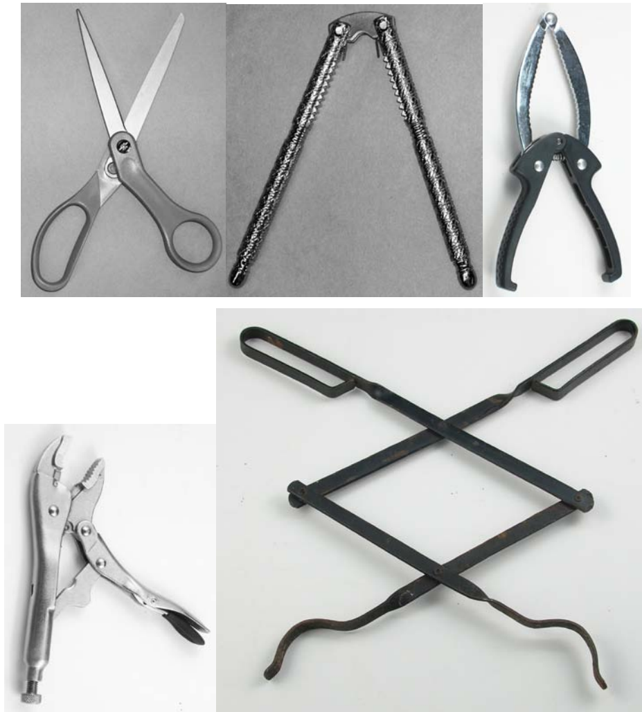
Figure 1: Sample mechanisms for modeling. Top row: scissors, nutcracker, jar opener; Bottom row: vise grips, fireplace tongs
