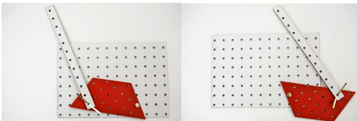
Figure 3: Showing how the input can control the lever moving it to other positions Use Post-Its™ or markers to label the two pivots in different colors, such as red for the fixed pivot and green for the floating pivot . Operate the mechanism so the whole class can see it, and ask:
