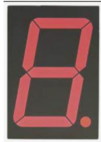
Seven-segment display (left) and 14-segment display (right)
